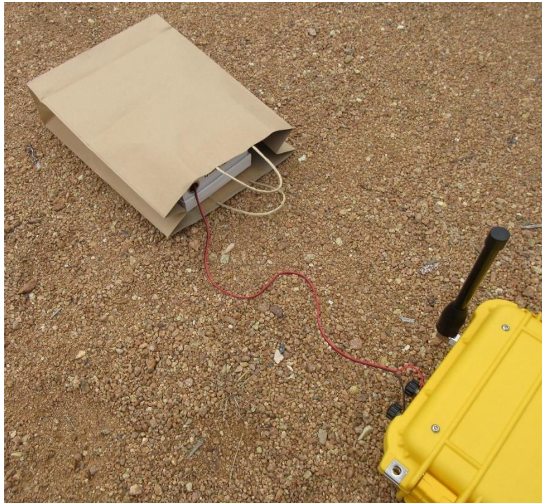
Figure 1.1 ExploSim Transmitter connected to training IED
